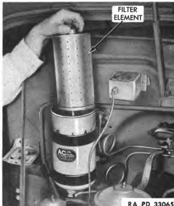
Figure 29—Oil Filter Element Replacement
