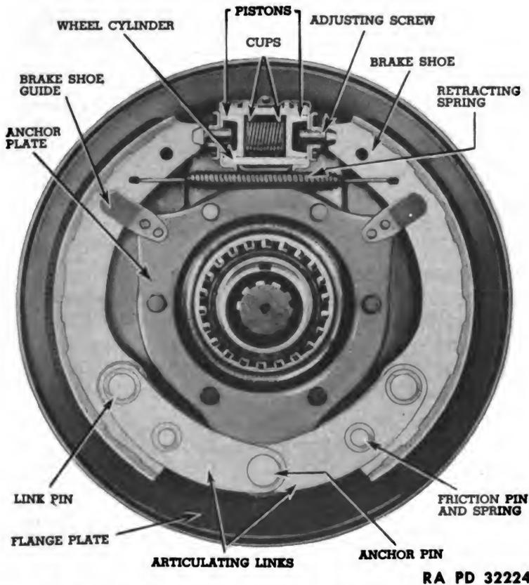
**Figure 103—Electric Trailer Brake Adjustment**
