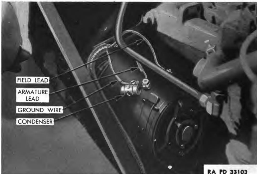
**Figure 72—Generator Condenser**
