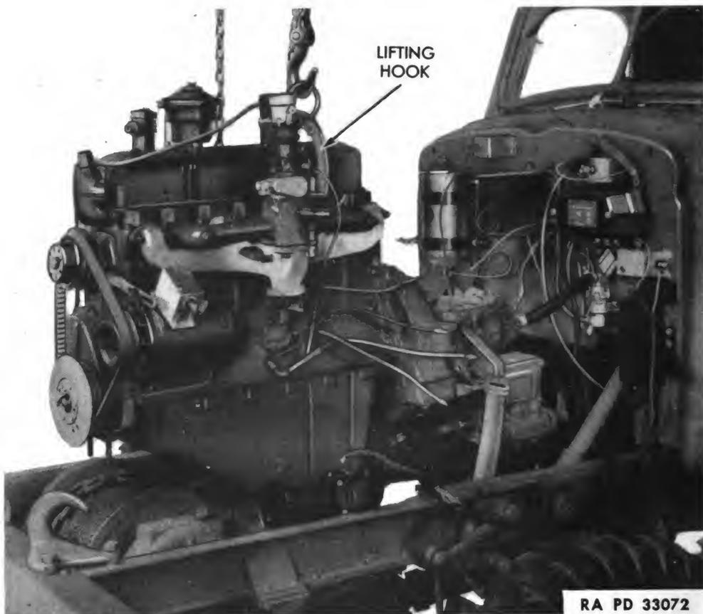
**Figure 32—Engine Assembly Removal**
