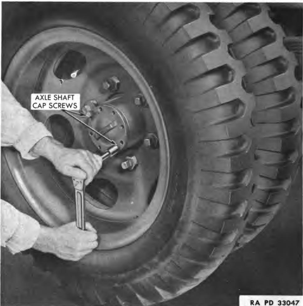
**Figure 87—Pulling Axle Shaft from Hub**
