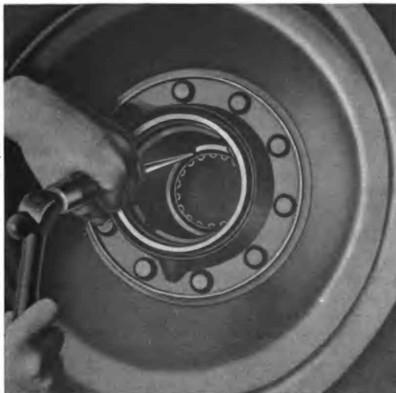
Figure 111—Removing Outer Bearing Snap Ring
