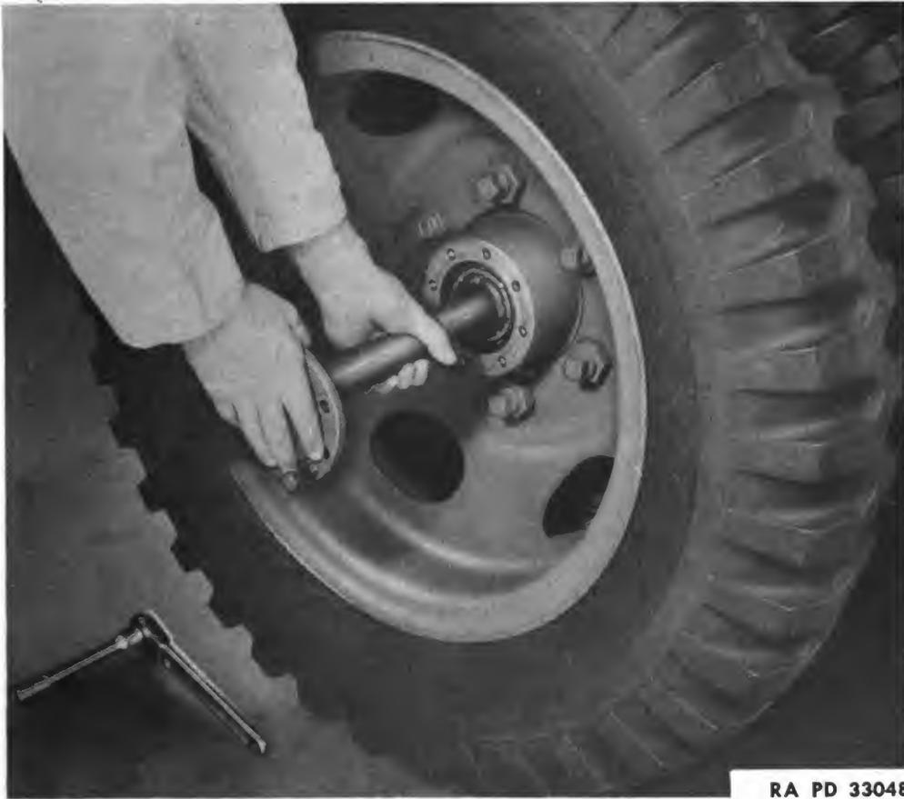
**Figure 88—Replacing Axle Shaft**
