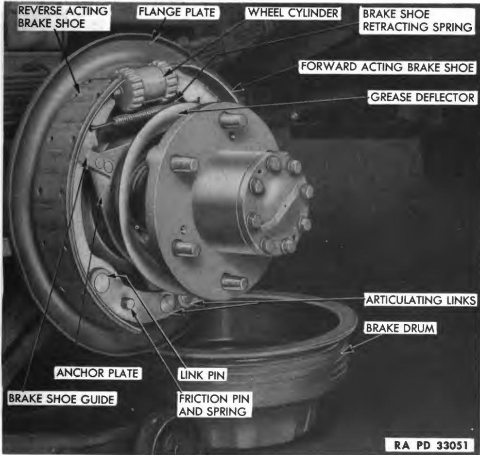
**Figure 100—Brake Construction, Rear Wheel**
