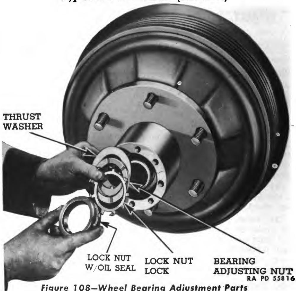
Figure 108—Wheel Bearing Adjustment Parts
